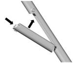
Now push the top part of the battery into the frame, until you hear the battery lock into position, and push the limiting stopper to keep the battery from dropping.
