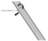
Then push the limiting stopper up to release the second locking mechanism and hold the two sides of battery to pull the battery.
